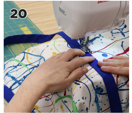
20. Topstitch the strap on both sides from the 4 1/4" line to the end.
